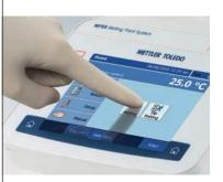
One Click™ determination is as simple as it sounds: all you need to do is press a button to start your measurement. Clicking the "Home" button on any menu takes you directly back to the initial screen.
