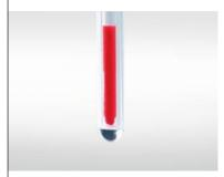
The slip melting point is the melting point of waxy solids and is defined as the temperature at which a sample has softened sufficiently to rise in an open capillary tube. It is used to characterize cosmetics, fats, and other substances with a waxy consistency.
